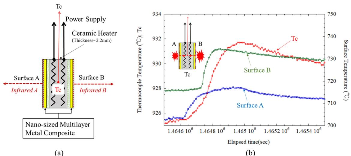
Figure 1. Evidence for surface heat release reaction; (a) Measurement points of Tc and Surface Temperature A and B, (b) Heat release reaction occurred at the surface A at first and afterwards at the surface B. Their heat bursts propagated to the Tc.
