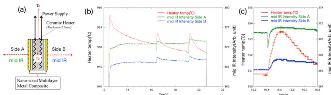
Fig. 1 (a) Schematic diagram of the experiment (b) Time evolution of Heater temperature, mid-infrared intensity (c) Enlarged view of the second heat burst.
