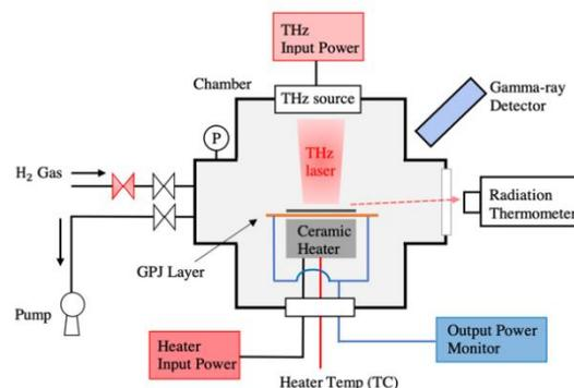
Fig 2. A schematic of the experimental setup.
