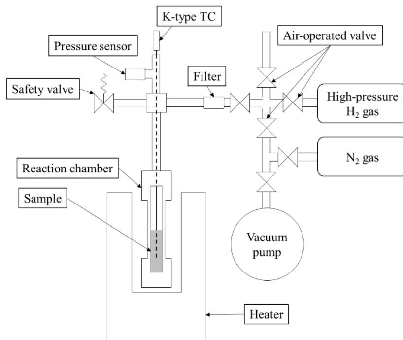
**Fig. 1.** Reaction system for experiments with high-pressure hydrogen gas
