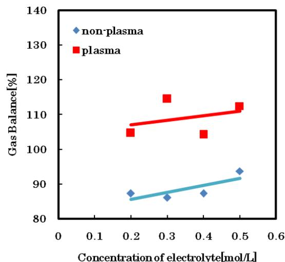
Fig 2. Dependence of gas balance on concentration of  $K_2CO_3$  at 90V
