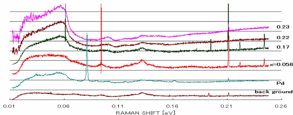
Fig.1 Raman spectra of PdH<sub>x</sub>.
