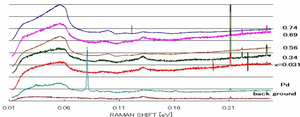
Fig.2 Raman spectra of PdD<sub>x</sub>.
