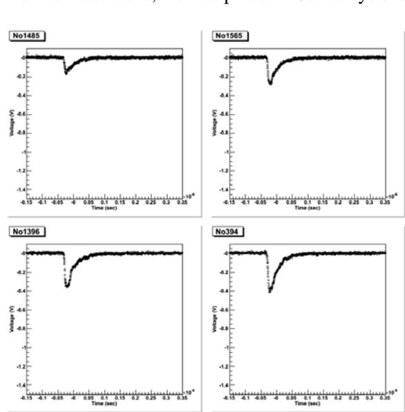
Fig. 1 Pulse shapes of 5.5MeV  $\alpha$  particles from  $^{241}\text{Am}$  checking source.
