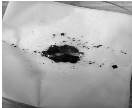
**Fig.6** Burning facial tissue due to the heat from the Pd deuteride. The time behavior of deuterium loading to this sample is plotted in Fig.3.
